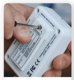
Install batteries and close cover with screwdriver
